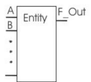
Architecture for this entity is created with Simple Signal Assignment Statement (SSAS).
