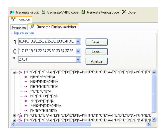
After minimization process, function tab will display "Minimization result" section, then you will be able to use actions for generating Circuit, VHDL or Verilog codes based on result of minimization.
