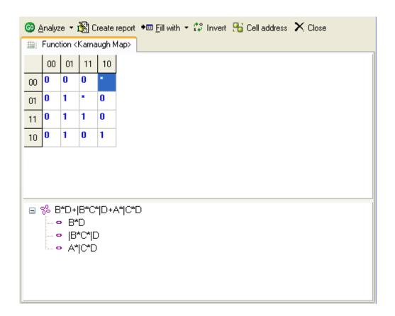
After analyze of Karnaugh Map you will be able to use "Create report" action, which quickly and easily make detailed report of minimization process. Also you can open appropriate function tab and generate Circuit, VHDL or Verilog code.
